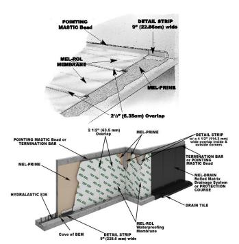
Inspect and Repair ... A thorough inspection should be made before covering and all necessary repairs made immediately. Tears and inadequate overlaps should be covered with MEL-ROL LOW TEMP ... slit fish mouths and patch. Seal edges of all patches with POINTING MASTIC. Where applicable, horizontal applications can be flood-tested for 24 hours. All leaks should be marked and repaired when membrane dries.
